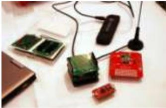
Component parts of the PocketQube including PCB from Newbury Electronics\*
