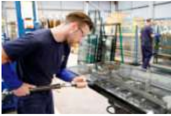
IG Units being manufactured at the St Austell production plant*
