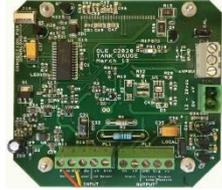
The completed gauge C2020 & associated PCB. Higher res image available on request.
